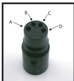
1) Locate the 4-pin rubber plug (R4) which plugs into the large plug on the front panel of the Cox-Box. The receptacle is in the shell and connects the wiring harness to the Cox-Box. Carefully snip the zip-tie that is securing the wires to the R4 plug.
