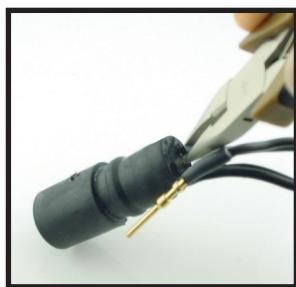
2) Using the pliers, hold the wire end of the sensor pin and carefully pull the stroke rate pins out of the R4 one at a time. They are the pins labeled 'A' and 'D' (be careful not to damage the two other pins). If the wires should come loose from the pins during removal, carefully pull the pins out separately.
