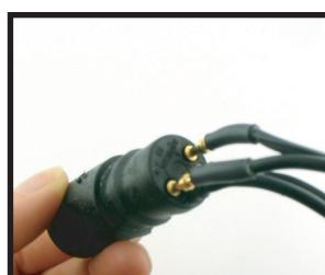
4) Position the new seat sensor pins into holes 'A' and 'D'. It does NOT matter which of the stroke rate holes the stroke rate pins are inserted into.
