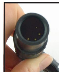
6) Check to make sure that the new pins should be even with the existing audio pins ('B' and 'C').
