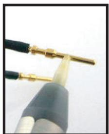
3) Apply Nyogel to the new pins and into the corresponding holes.
