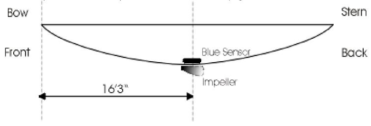
**Very important:** The BLUE speed sensor DOES NOT sit directly above the impeller, it must cut the magnetic field & so should sit either ACROSS the hull mount OR just in front or behind the hull mount, as per the diagrams below.
